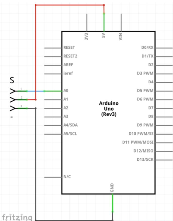
For the successful connection of the Heart Pulse Sensor with the Arduino board, it is necessary to connect 3 connecting pins. We connect the extreme pin S with the A0 pin, the middle pin with a 5 V Arduin pin and the extreme pin "-" with the Arduin ground.
